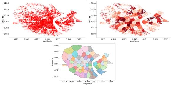
Fig. 1. Spatial Partitioning Approach for the example of Cologne (Germany)
